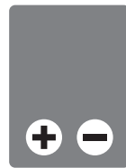
Image 2 Pole terminals layout (battery capacity over 110 A/h)
